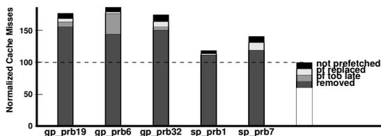
Figure 13. Breakdowns of cache misses to understand the tuning curves of the join phase
