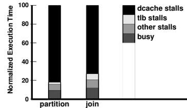
Figure 1. Execution time breakdown for hash join.
