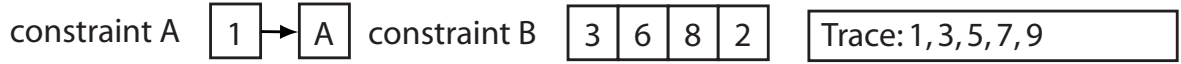
Figure 7: Access dependency. This figure shows an access dependency. Sequential constraint B is dependent on placement constraint A because constraint A affects a block which precedes a block in constraint B.
