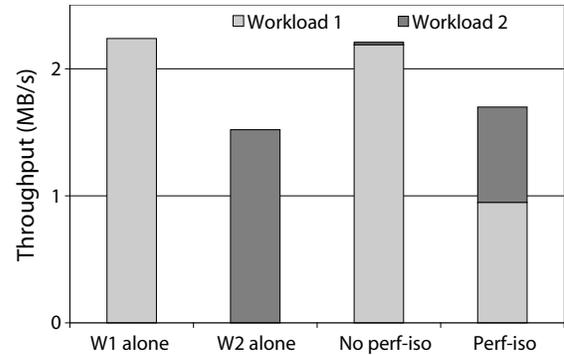
Figure 7: **Quanta-based scheduling support for two random-access workloads.** The standard deviation is at most 0.02 MB/s for these bars.
