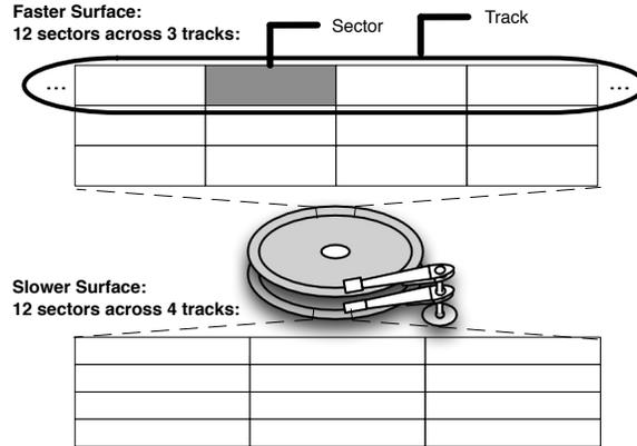
Figure 1: **Adaptive zoning of disk drives.** The same area of different disk surfaces within a drive are formatted according to the physical properties of the disk head. Each of the surfaces pictured have equivalent areal density, although the top surface is faster because it accommodates more sectors per track over fewer tracks, while the bottom surface has a narrower disk head that requires fewer sectors per track but allows for more tracks.
