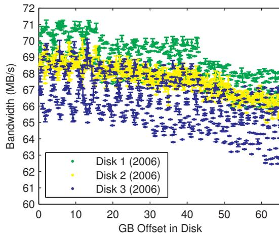
Figure 3: **A closer look at inter-disk behavior with adaptive zoning.** The first 64 GB of the 2006-era disks show that the same logical blocks have consistently different bandwidths across disks (error bars are shown with standard deviation).
