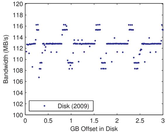
Figure 4: **A closer look at intra-disk behavior with adaptive zoning.** A smaller block size of 12 MB for the 2009-era disks clearly distinguishes between bandwidth differences across disk heads and surfaces.
