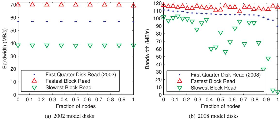
Figure 5: **Disk drive performance statistics.** Reading the first quarter (9 GB) of an older 2002-era drive that doesn't implement adaptive zoning shows identical behavior across 9 disks. However, reading the first quarter (250 GB) of a modern 2008-era drive with adaptive zoning produces a 21 MB/s spread of average bandwidth, and the minimum and maximum values for each 128 MB block also have considerably more variation across otherwise identical-model disks.
