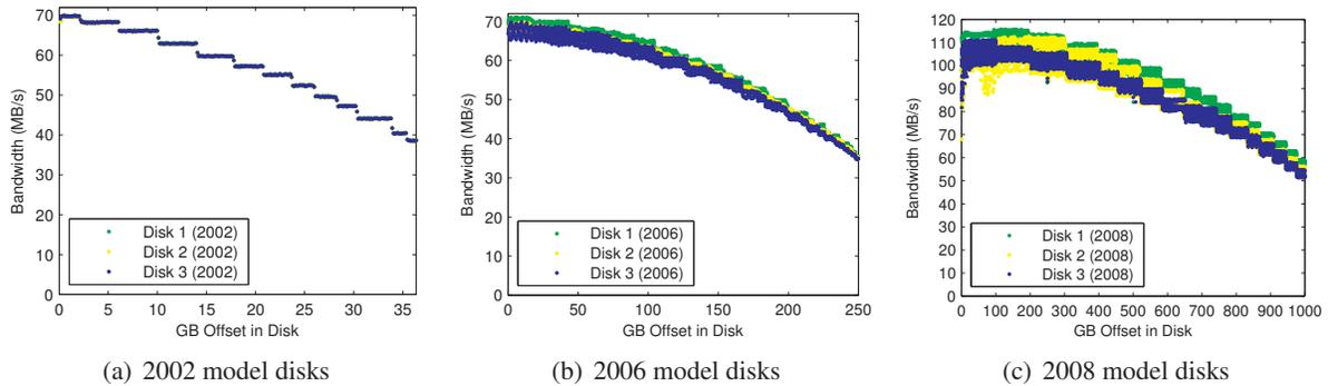
Figure 2: **Evolution of disk behavior over time.** Comparing 128 MB block read bandwidth for a representative sample of 3 sets of identical-model disks, from 2002, 2006, and 2008, demonstrates both a large increase in capacity and a growing trend of heterogeneity within each set of disks. Results for disks within a set are plotted atop one another.
