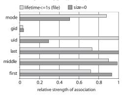
Figure 2: The relative strength of the correlation between the properties "lifetime (lftmd) is one second or shorter" and "size is zero" and several file attributes (as indicated by the chi-squared values) for one day of each trace. The chi-squared values are normalized relative to the attribute with the strongest association. The last, middle, and first attributes refer to components of the file name, as described in Section 5.
