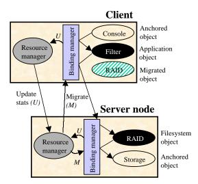
Figure 2: The architecture of the ABACUS migration system. An application is broken up into a number of migratable objects. Calls between the objects are redirected by binding managers that know where the objects are currently running. Binding managers also inform resource managers about the resources consumed by the objects. The resource managers use this information to reevaluate how objects are partitioned among clients and servers.
