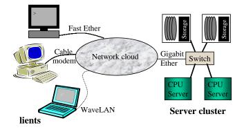
Figure 1: Users running data-parallel applications across the Internet. The data stores are on server clusters, which, compared to monolithic machines, flexibly support different kinds of concurrent workloads, are easier to upgrade, and have the potential to support independent node faults. Our client machines, in contrast to the traditional view, are active collaborators with the clusters in providing the end-result to the user.
