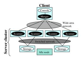
Figure 4: The decomposition of a data-parallel application into scanning and merging objects. The dataset is stored across two storage nodes. The scanning object is computationally expensive so there are more scanning nodes than storage nodes. When the scanners aren't costly, ABACUS would configure the system to look like one of the examples in Figure 5.
