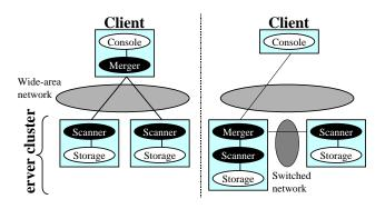
Figure 5: Adapting the merge object location. On the left, the wellconnected client is running the merge object, offloading this work from the contended server cluster. On the right, the client has relatively poor connectivity, and to avoid this "last-hop" network bottleneck, ABACUS migrates the merge object down to one of the nodes in the server cluster.
