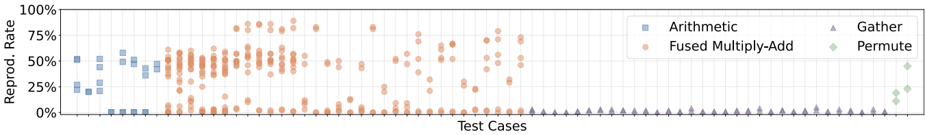
Figure 9. Reproduction rate of the test cases with identical inputs. Each data point is a processor core that detects SDC with the corresponding test case. We show test cases for different operation types in different colors.
