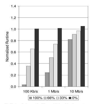
Mozilla install times with different Jukebox hit-ratios at 100 Kb/s, 1 Mb/s, and 10 Mb/s with 100 ms, 10ms and no added latency respectively. Each bar is the mean of three trials with with the maximum standard deviation observed as 1%.
