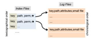
Figure 3: Column-style stores index and log tables separately. Index tables are kept in LevelDB which contains frequently accessed attributes for file lookups and the pointer to the location of full file metadata in the log file.
