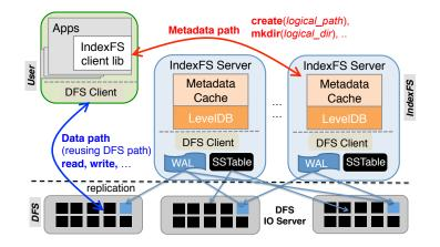
Figure 1: The IndexFS metadata system is middleware layered on top of an existing cluster file system deployment (such as PVFS) to improve metadata and small file operation efficiency. It reuses the data path of the underlying file system and packs directory entries, file attributes and small file data into large immutable files that are stored in the underlying file system.
