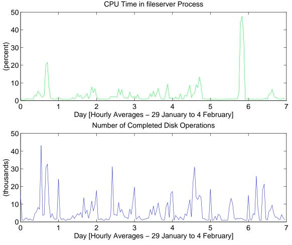
Figure 3 - CPU and Disk Utilization
