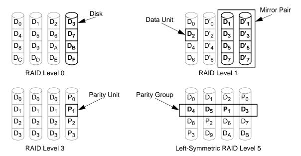
Figure 1 RAID Levels 0, 1, 3, and 5. This figure depicts the data layout and redundancy organizations for the most prevalent RAID levels using an array of four disks. *Data units* represent the unit of data access supported by the array. *Parity units* represent redundancy information generated from the bitwise exclusive-or (parity) of a collection of data units. The redundancy group formed by a parity unit and the data units it protects is commonly known as a *parity group*.
