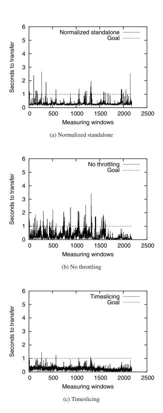
Figure 1: Bandwidth guarantee adherence over time for a dedicated disk and two of the schedulers
