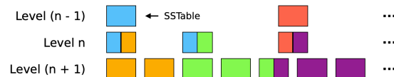
Fig. 24: Units of work in LSM compaction. When declaring compaction, we strive to declare clean cuts of work such as the orange files and the purple files instead of overlapping work such as the orange files and the blue files.
