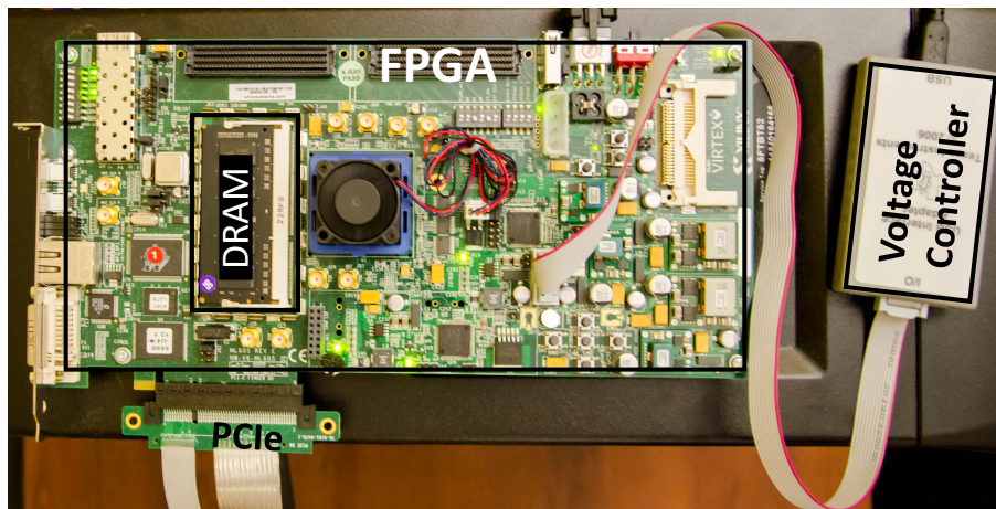
Fig. 3. FPGA-based DRAM testing platform.
